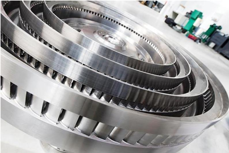
**1. One disk, two stages.** Exergy's radial outflow turbine, designed for binary Organic Rankine Cycle systems, is driven by both high- and low-pressure vapor across a single disk. The company says this approach is both more efficient and less expensive than conventional designs. *Courtesy: Exergy*
