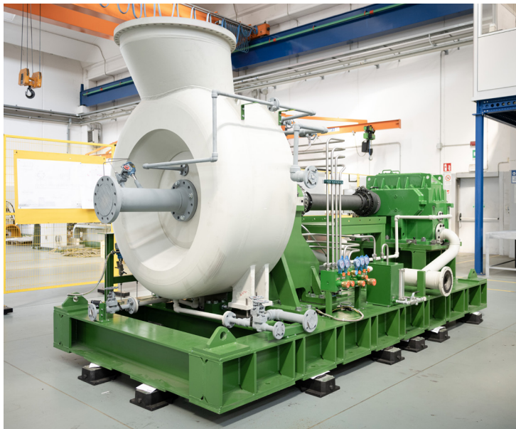
An Exergy Radial Outflow Turbine in the workshop.
